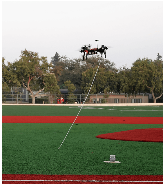
Fig. 12 Manoeuvring with the Tether Deployed. The large mass of the probe coupled with the long tube length means the probe lags significantly behind the vehicle and even small manoeuvres at low speeds can introduce significant swinging.
