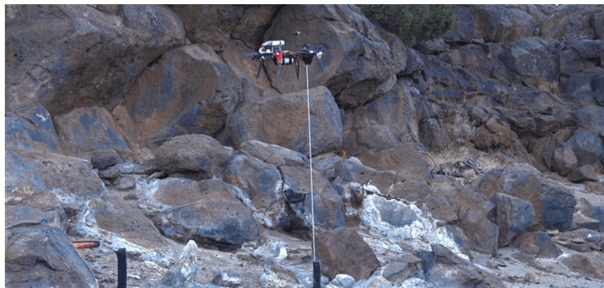
Fig. 16 Capturing Gas from a Capped Fumarole at Basalt Fumarole
