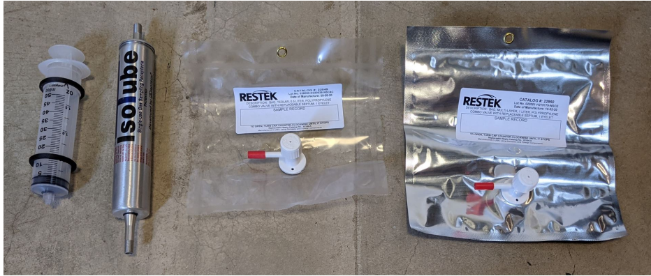
Fig. 5 A Selection of the Sample Canisters. Left-to-right: Syringe (50 ml), IsoTube (100 ml), Tedlar Bag (500 ml), Multi-Layer Foil Bag (1 000 ml).
