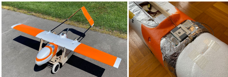
Fig. 9 Example of a GPS antenna ground plane. Note the continuation of the ground plane towards the wing mount.
