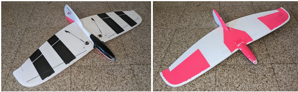
Fig. 7 Painting aircraft in bright colours with different patterns on the top and bottom helps the pilot maintain orientation of the aircraft at long distances
