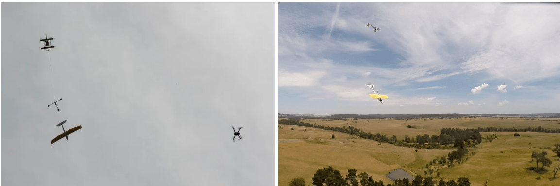
Fig. 6 Dropping aircraft from a tether can be used when a conventional launch is impractical [2]
