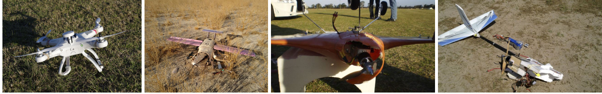
Fig. 17 Crashes. Causes from left to right - not confirming correct throttle levels set on transmitter for UAV handover, not accounting for the loss of thrust with altitude, not capturing the forward shift of the aerodynamic centre during high-thrust, low airspeed conditions for a blended wing body, aero-elastic flutter of the elevator during a dive leading to loss of control.
