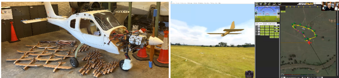
Fig. 18 Student projects using UAS. The fleet of RC models built by students when constrained from building the kitplane due to COVID-19 restrictions in 2021 (left) and RC model being flown by autopilot (Mission Planner) in simulation (RealFlight 9.5) (right).
