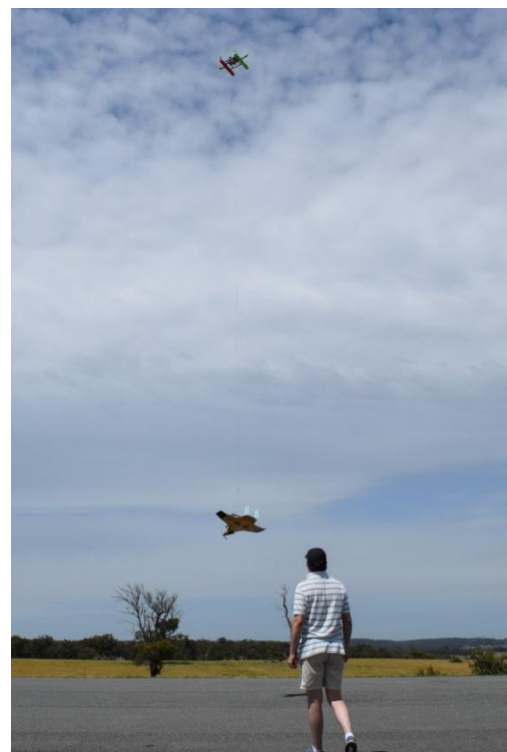
(b) The Sky-Crane Lifting the Blended Wing Body Experimental UAV
