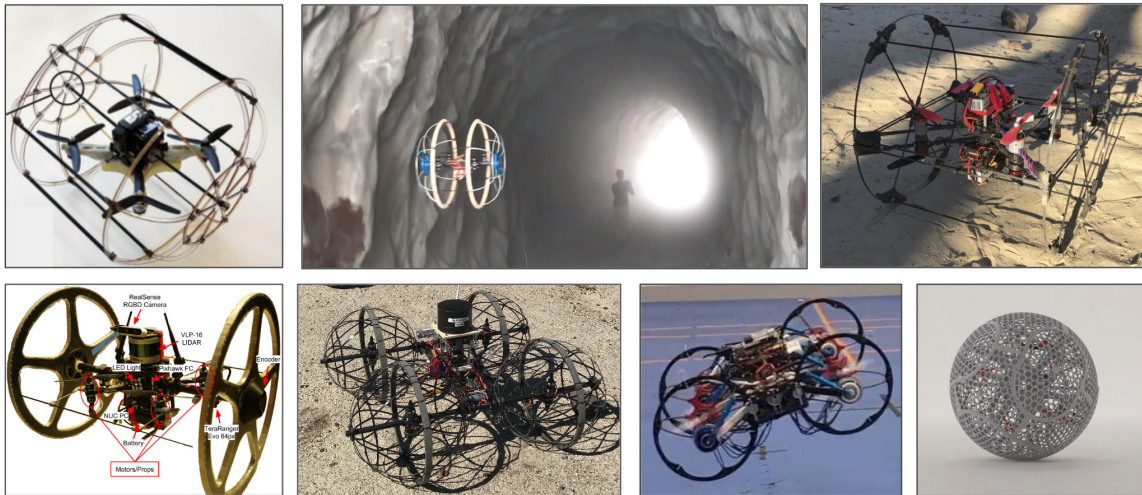
Figure 50. Hybrid platform hardware evolution (top row, left to right) pre-challenge Hytaq design (Kalantari and Spenko, 2014), modular hybrid vehicle (Agha-mohammadi et al., 2020), (bottom row, left to right) autonomous rollocopter (Fan et al., 2019; Lew et al., 2019), DrivoCopter (Kalantari et al., 2020), BAXTER (Choi et al., 2020), spherical rollocopter (Sabet et al., 2020, 2019).
