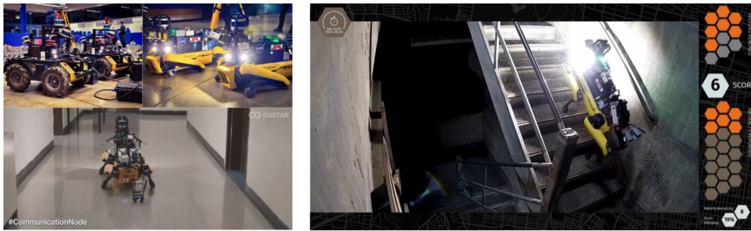
Figure 65. Robot team deployed at the Urban Circuit event. Left: Robot fleet and communication node deployment. Right: A snapshot of Spot stair climbing (DARPA TV).
