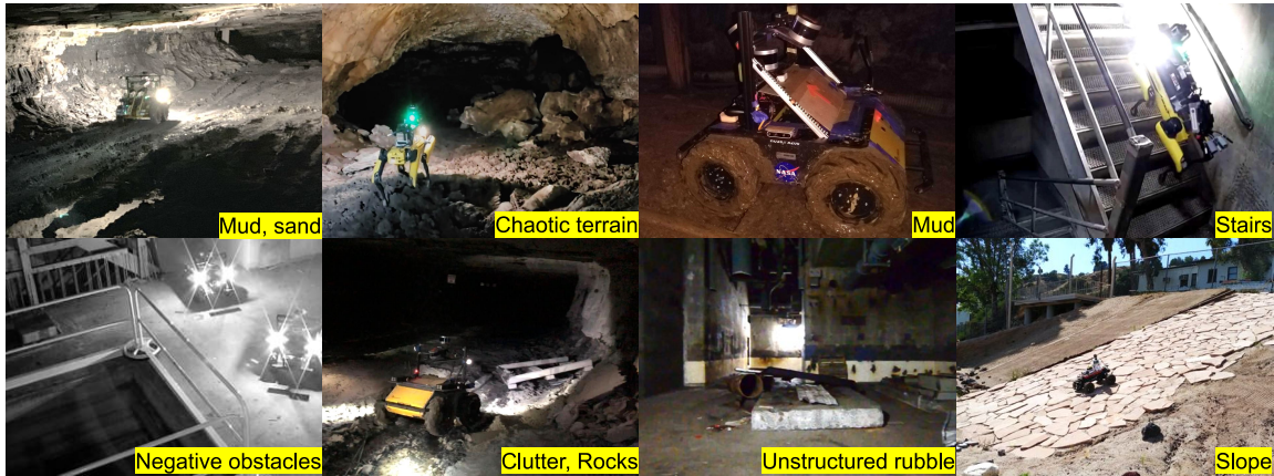
Figure 22. Mobility-stressing elements commonly found during testing in various tunnel, urban, and cave environments, including 800 ft underground at Arch Mine in Beckley, WV, Valentine Cave at Lava Beds National Monument, CA, Satsop power plant in Elma, WA, and Mars Yard at JPL, Pasadena, CA.
